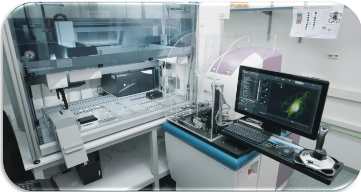
Figure 1 - The Hermes 24/7 system at the Gerst lab, Weizmann Institute. The system is integrated to a Freedom Evo liquid handler by Tecan.
